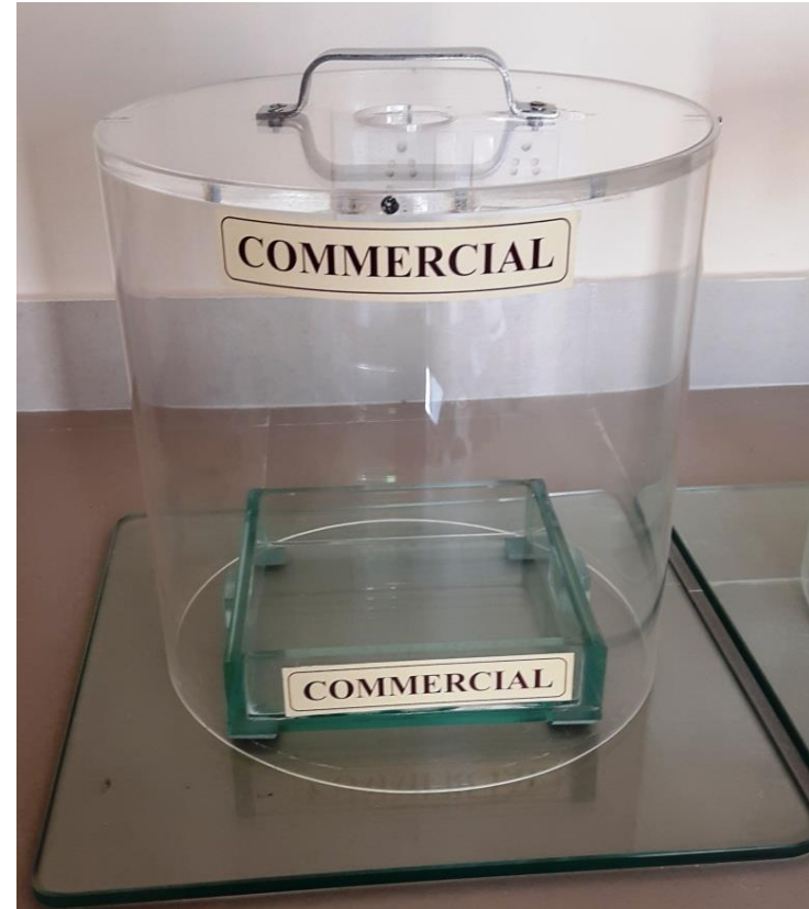
Brick Efflorescence Testing Apparatus. IS:3495, Part-III., Model: CE-SP001
