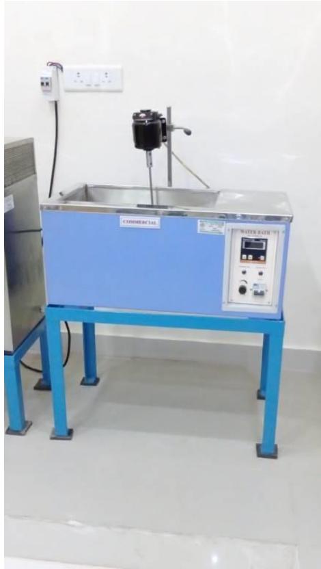
Constant Temperature Water Bath, Electrically Heated. Temperature from ambient to 80deg.C. Size (18"x12"x7"). Model: CE-HC164
