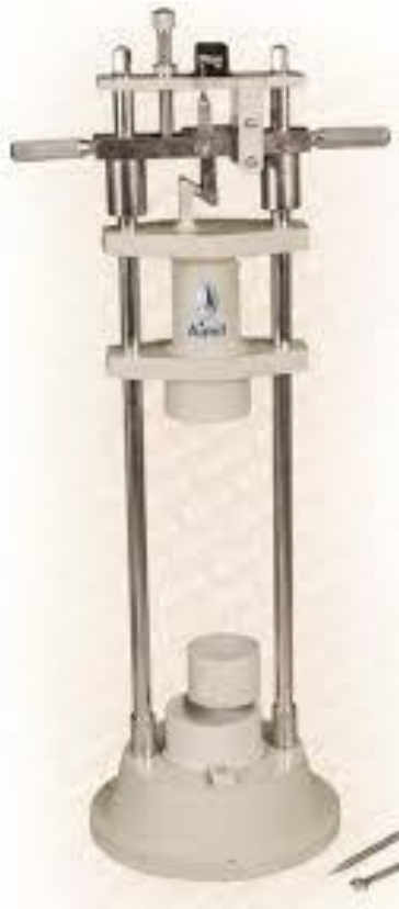
Aggregate Impact Tester, IS: 2386 (IV) with Automatic Blow Counter., Model: AIM-456
