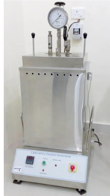
Cement Autoclave, Analog with Pressure Gauge & Digital temperature Controller, Model: AIM-408-2
