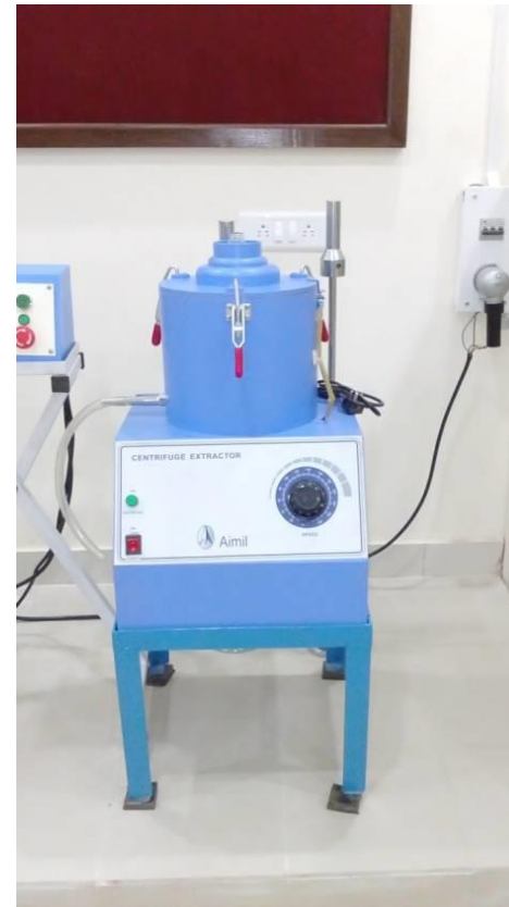
Centrifuge Extractor, Electrically Operated, Cap.: 1500g. (ASTM D2172) AASHO T- 58, T-164) , Model: AIM-563-1
