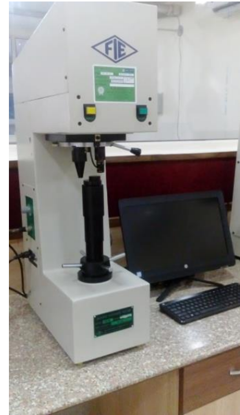
Computerised Vickers Hardness Tester Model: VM-50 PC, Total loads: 5,10,20,30,50 kgf.
