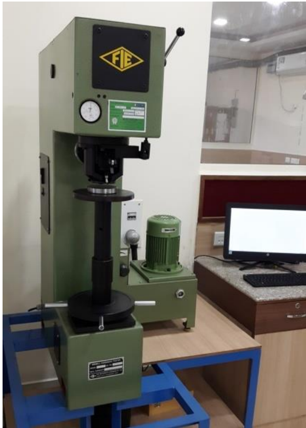
Computerized Brinell Hardness Tester, Model B-3000(PC), Total loads 500 to 3000 kgf in stages of 250 kgs
