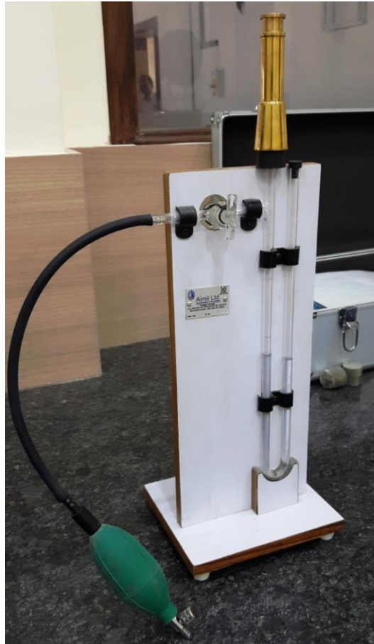
Air Permeability Apparatus, Blain Type, ISI mark, Model: AIM-390
