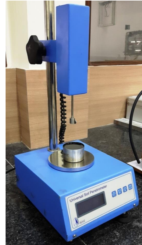
Universal Penetrometer, Digital Type New Type for Soil and Bitumen testing, Model: AIM-042-3
