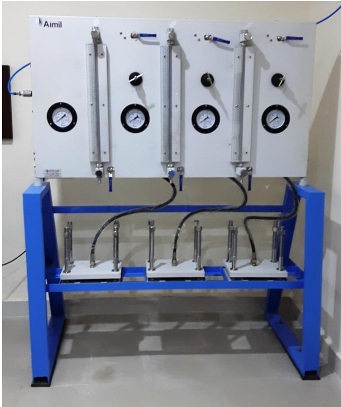
Concrete Impermeability Apparatus, 3 cell model for 150 mm cube as per DIN Std. Model : AIM-384.
