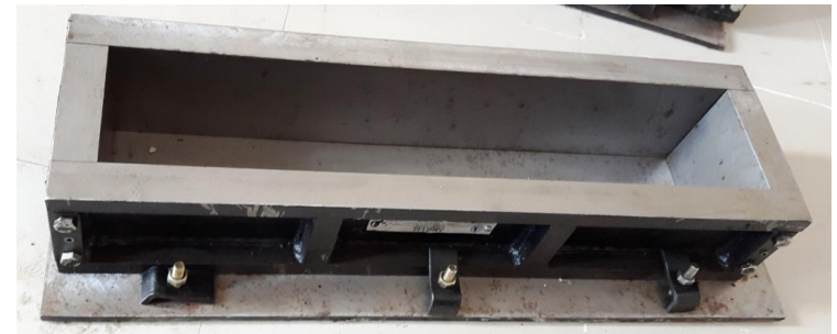
Cube, Cylindrical & Beam moulds
