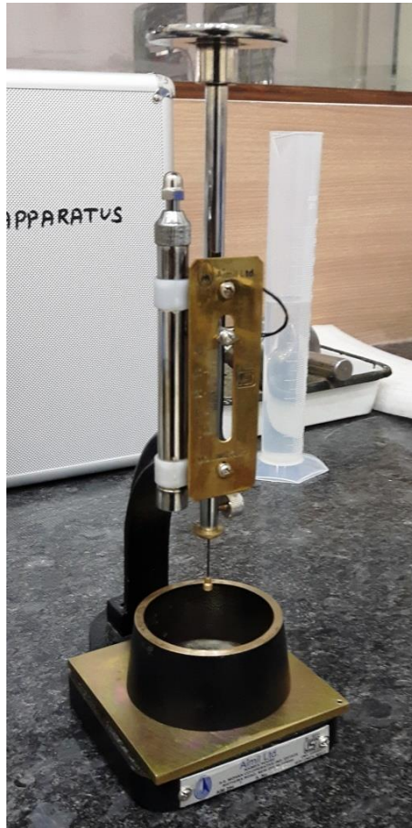
Vicat Apparatus with Dashpot ISI mark, Model: AIM-394
