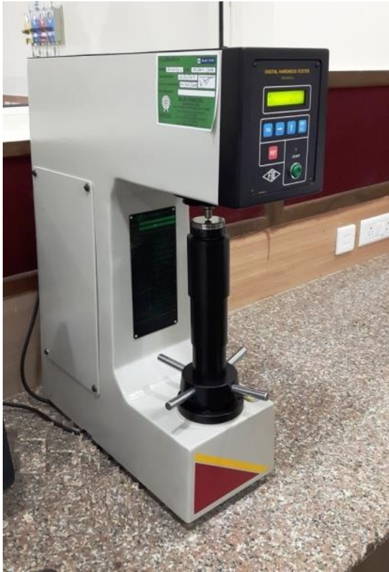
Rockwell hardness testing machine Model: RASNE-B3, Tests ; A , B & C Scale
