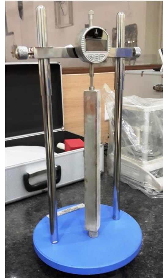
Length Comparator, Digital. Model: AIM- 374-1-DG
