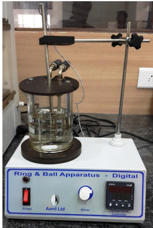
Ring and Ball Apparatus, Semi Automatic, IS:1205, Model: AIM-561-2
