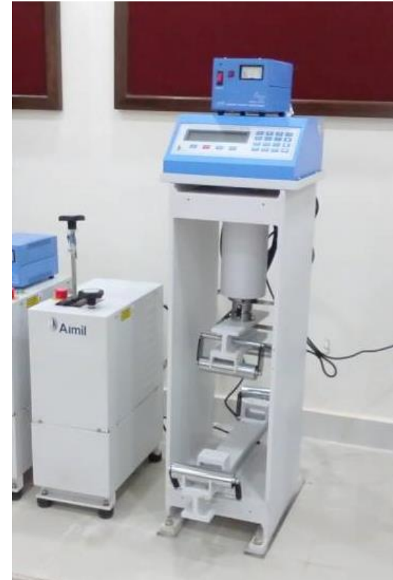
Digital Flexure Testing Machine, Capacity: 100kN, Model: AIM- 332-E-DG-1
